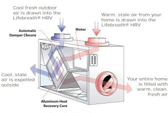
Heat from the indoor air is transferred via the aluminum core to the incoming fresh air stream
