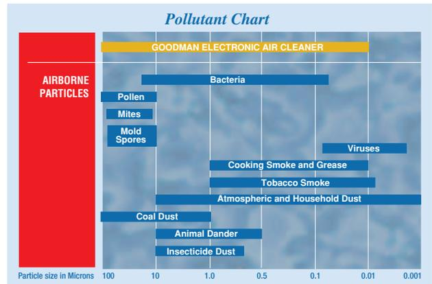
Environmentally-friendly, Lifetime Filter System removes harmful airborne pollutants as small as .01 micron (1/2,540,000 of an inch) in size.
