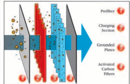
The furnace blower moves the dirty air throughout the house into the electronic air cleaner. The prefilter first removes all of the larger particulate matter. Smaller particles are then given a powerful positive electrical charge. These charged particles are then attracted to the grounded plates where they adhere like a magnet until washed away during cleaning.\* Finally the clean air passes through activated carbon filters for odor removal.
